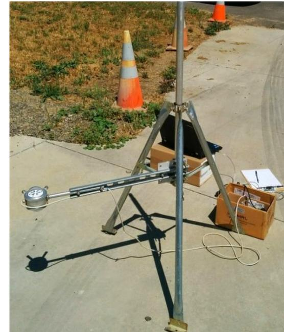
Albedometer with dual-pyranometer
